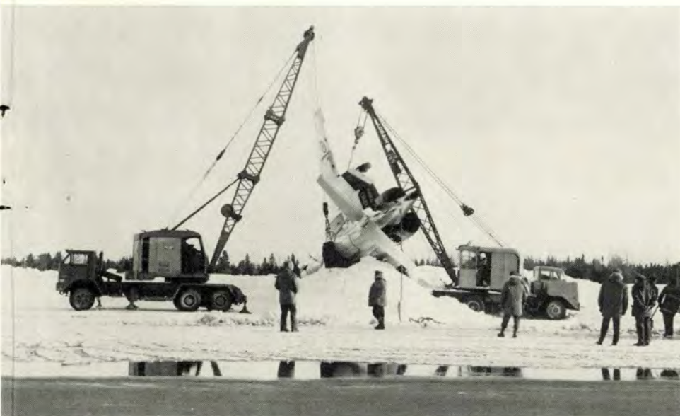
Pilot was not warned of compacted snow ridge on runway. Picture above shows result.
